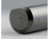
The Boron STC drill bit, made from tungsten-carbide, is designed specically for use on spot welds made for boron steel with tensile strength from 450N/mm2 - 1.580N/mm2. Triple fluted to spread the torque forces over a greater area, and special multi-layer coating is applied to help reduce friction.
