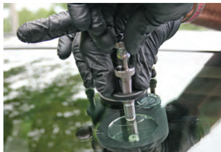
12. Screw injector plunger until it stops. DO NOT over tighten.
