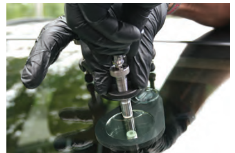
13. Begin your first pressure cycle. Hold barrel with off hand, pull back on plunger with other hand, rotate 1/4 turn clockwise, and gently lower into place.
