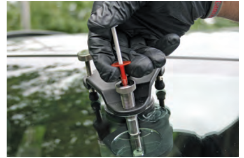
10. Make sure you get the resin to the bottom of the injector barrel. The white end seal must be filled with resin for a successful repair.
