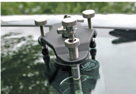
11. Put the injector plunger in the vacuum position. Pull back on the knob, rotate 1/4 turn clockwise, and lock in place. Ensure that the piston is retracted.
