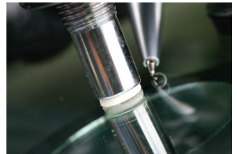
10. Make sure you get the resin to the bottom of the injector barrel. The white end seal must be filled with resin for a successful repair.
