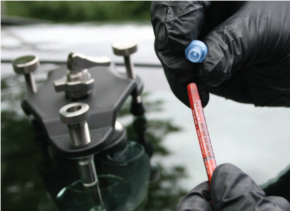
9. Load the injector with 1 syringe of fill resin.
